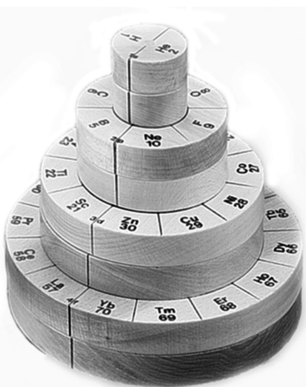
Figure 7. Periodic round table. Actual radii of the tiers = 1.5 in, 3 in, 4.5 in, 6 in. Height = 6 in. The nominal thickness of each disc (period) is 0.75 in and it is constructed of hardwood.
